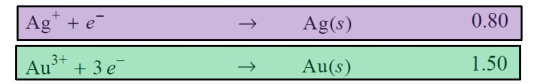
Cathode = reduction = gain e- = more + E Anode = oxidation = loss e- = more - E (less +)
